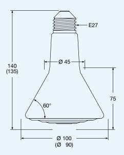
Figure: 68 Mounting dimensions and radiator dimensions () in mm
